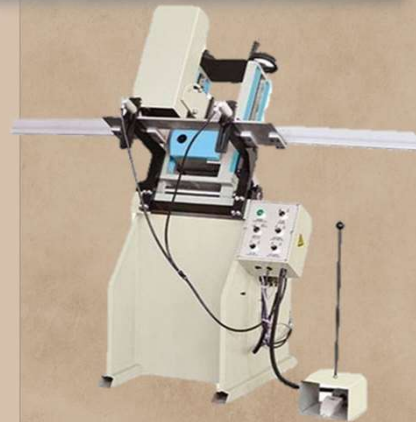
Water slot cutting M/c
